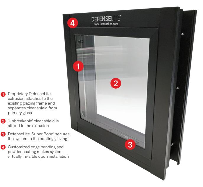
Each system is custom fabricated based on existing glazing conditions and installed by certified installers. Systems may utilize exotic plastics, polycarbonates and glass-clad shields depending on threat conditions and budgets. All-weather adhesives, high-performance films, mechanical anchors and other matirials may be used. shields install on the exterior or interior of existing windows and doors. Systems have been independently tested to meet forced entry and UL752 ballistic standards.
