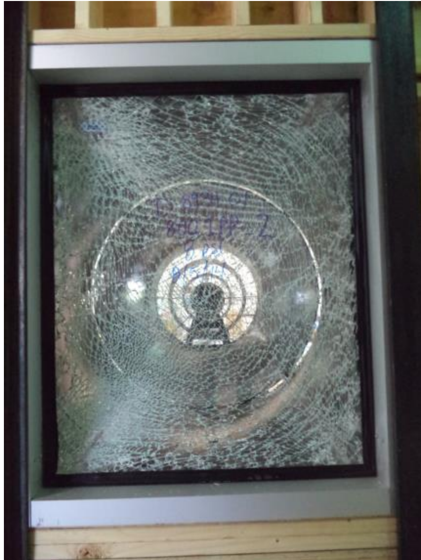
Photo No. 5 Post-test Specimen #2, Interior
