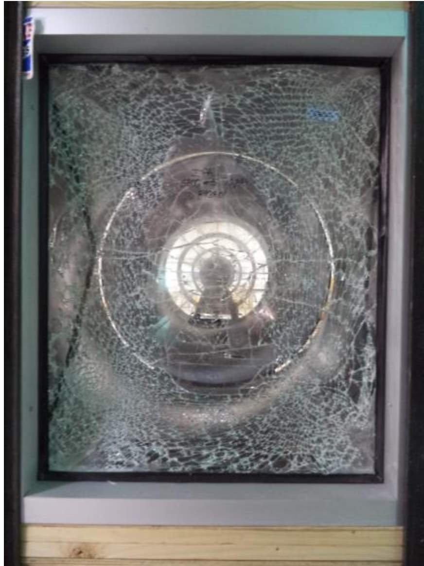
Photo No. 29 Post-test Specimen #10, Interior
