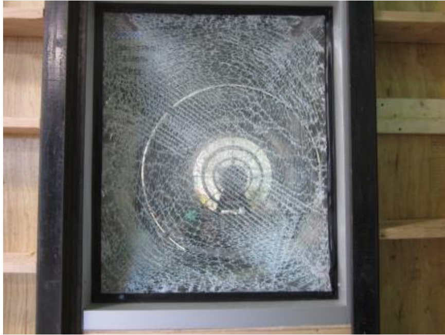
Photo No. 8 Post-test Specimen #3, Interior
