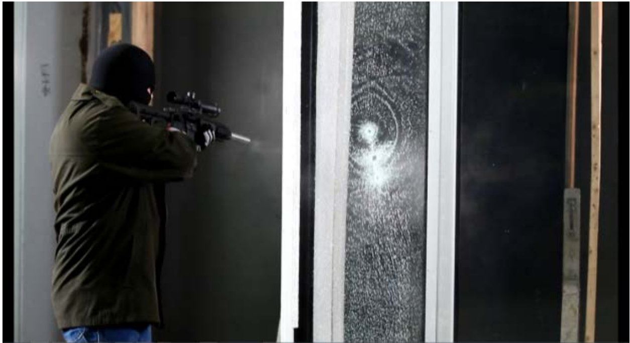
Test #4: 3M Ultra 800, Semi-automatic rifle attack, after 4 shots.
