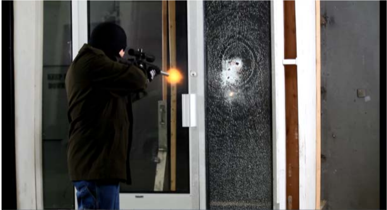
Test #3: 3M Ultra 800, Semi-automatic rifle attack, after 4 shots.
