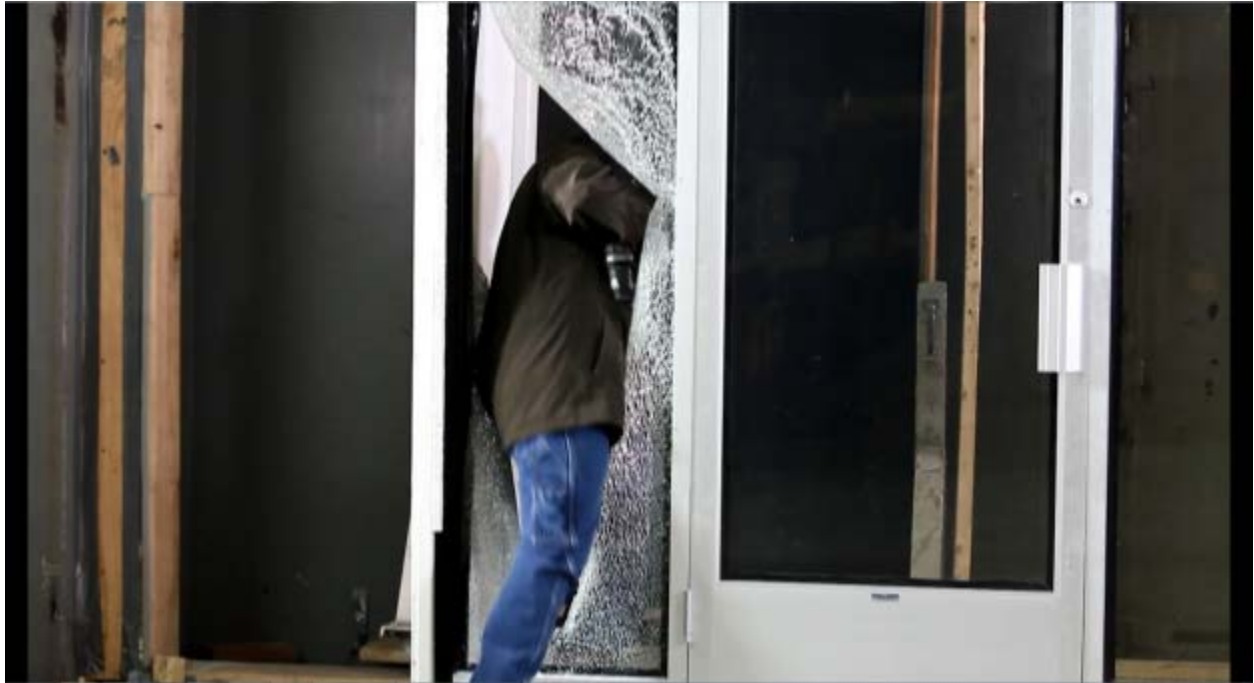
Test #4: Semi-automatic rifle attack, access gained after 43 impact and 48 seconds.
