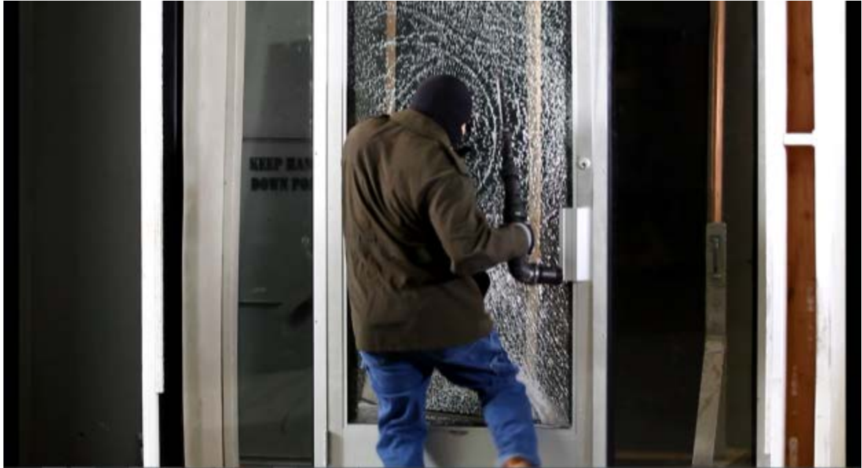
Test #5: Semi-automatic rifle attack, after 70 seconds.
