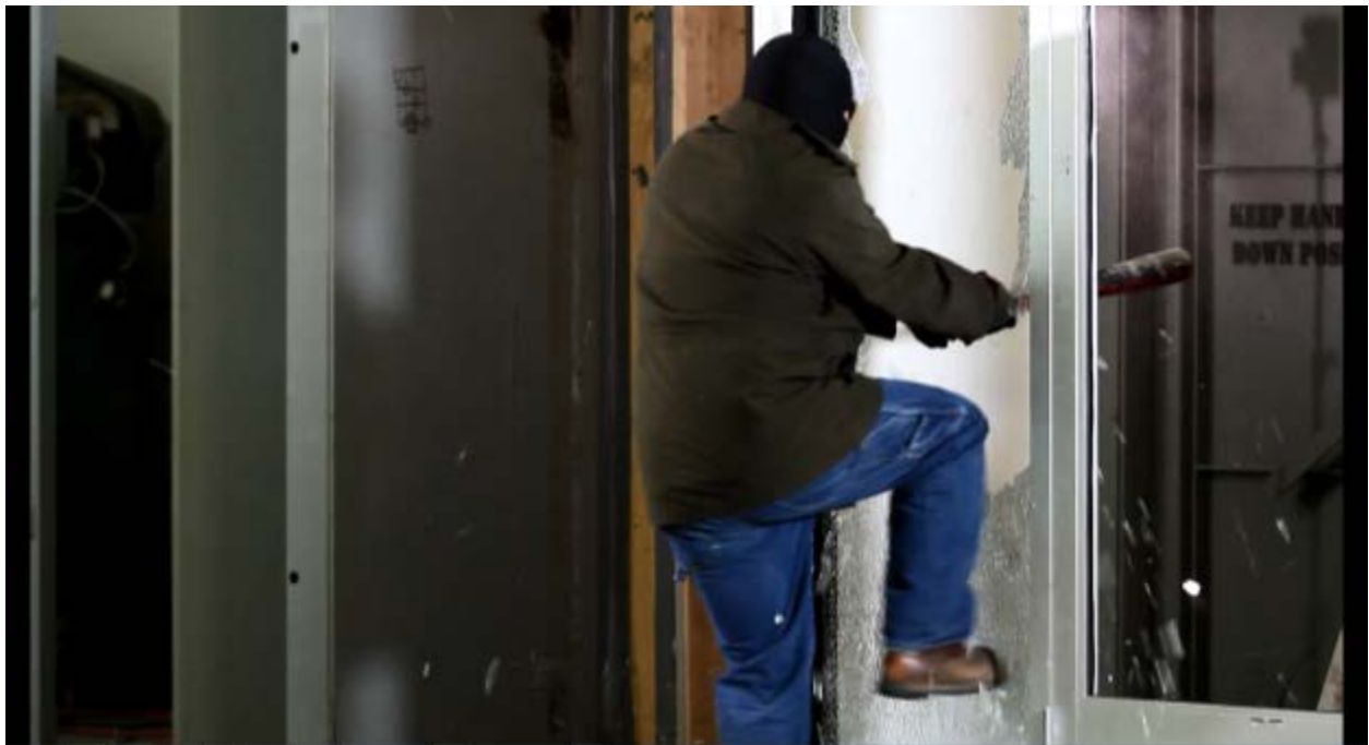
Test #6: Bat attack, NO FILM, access gained in 6 seconds.
