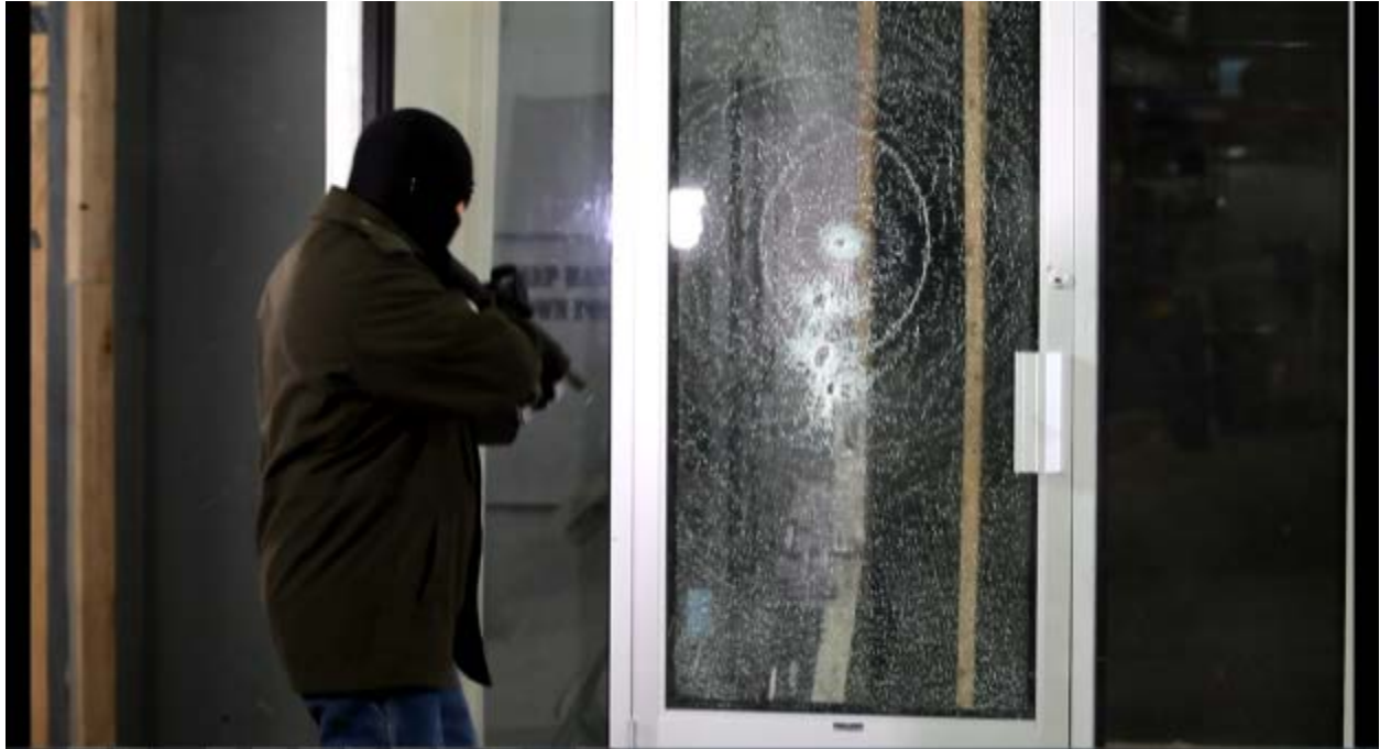
Test #1: 3M Ultra 800, Semi-automatic rifle attack, after 4 shots.
