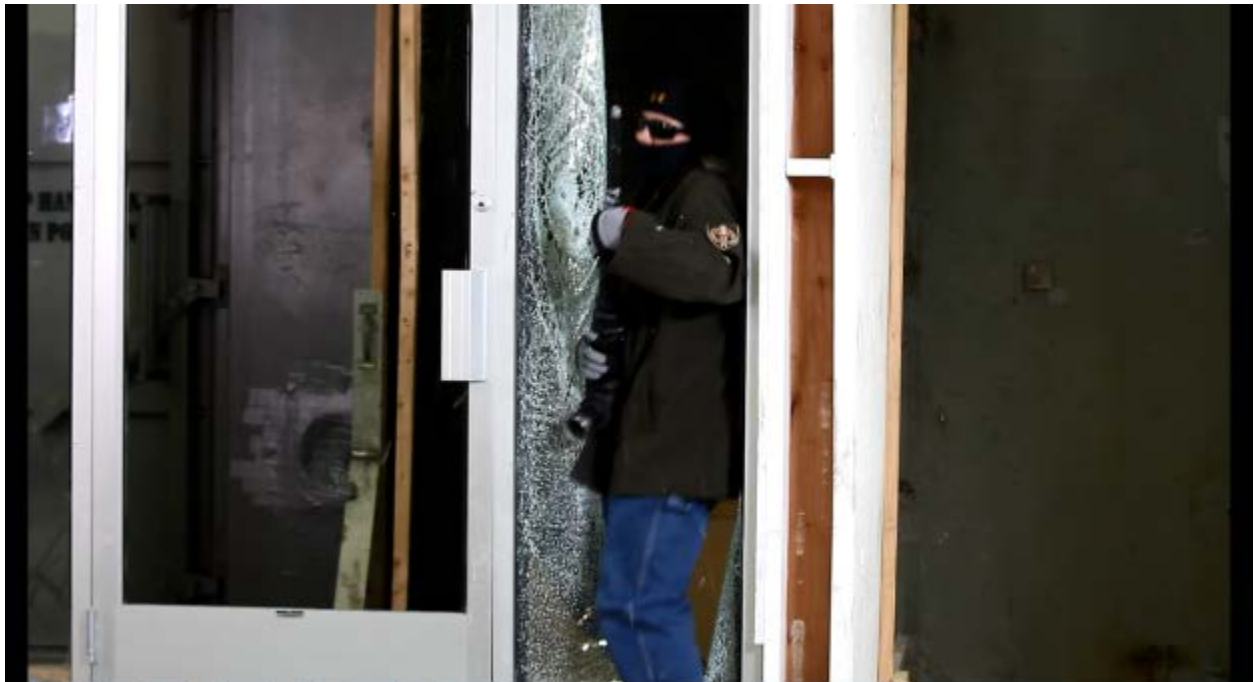
Test #2: Semi-automatic rifle attack, access gained after 38 impacts and 60 seconds.
