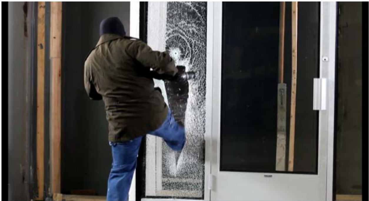
Test #4: Semi-automatic rifle attack, after 38 seconds.
