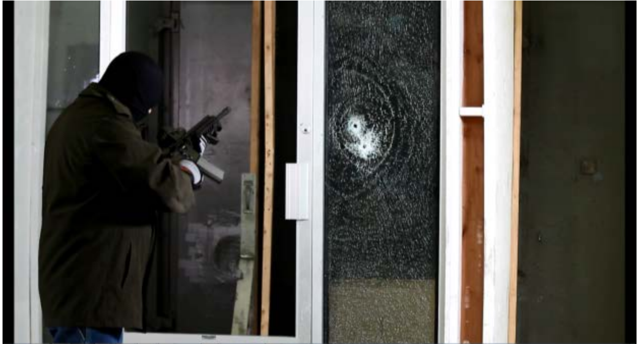
Test #2: 3M Ultra 800, Semi-automatic rifle attack, after 2 shots and jammed gun.
