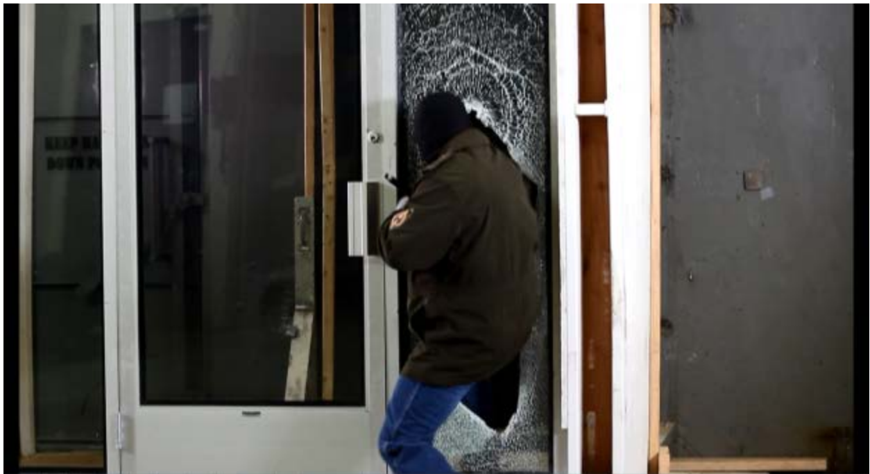
Test #3: Semi-automatic rifle attack, access gained after 45 impacts and 50 seconds.
