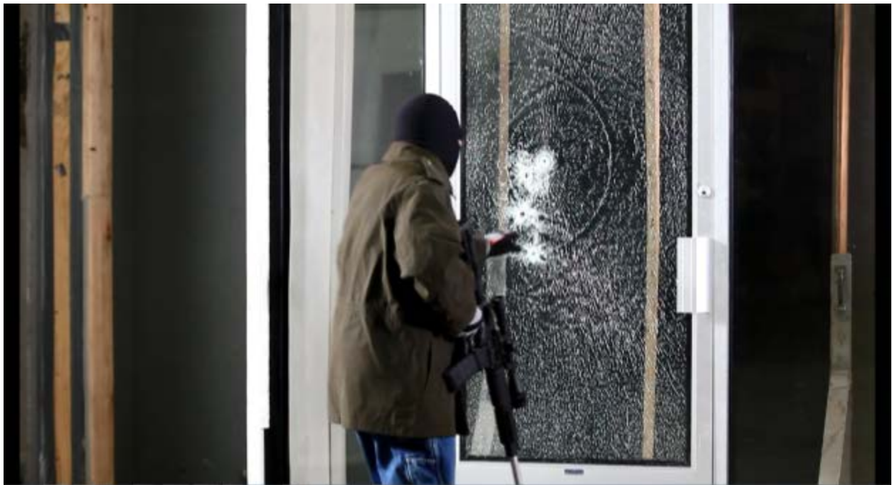
Test #5: Semi-automatic rifle attack, 3M Ultra 800 (interior) with Safety S70 Exterior (exterior).
