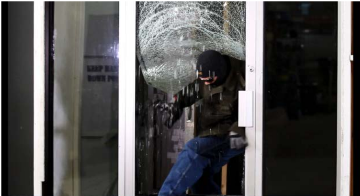
Test #1: Semi-automatic rifle attack, accessed gained after 33 impacts and 35 seconds.
