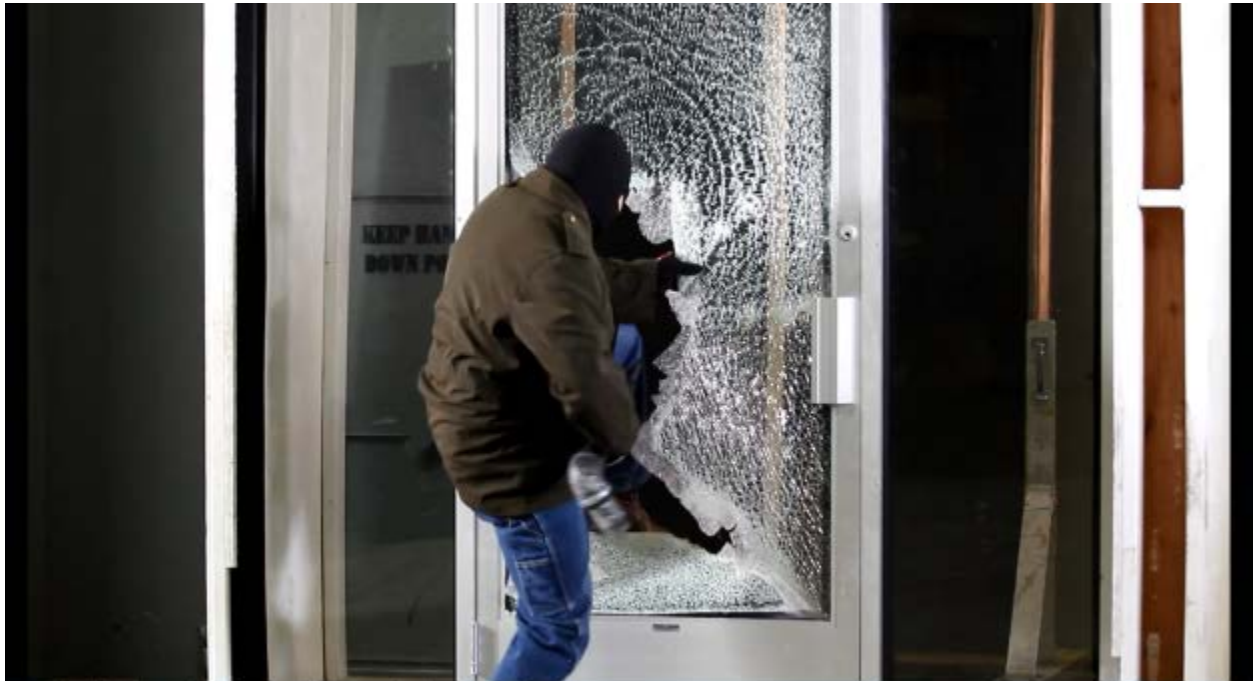
Test #5: Semi-automatic rifle attack, access gained after 70 impacts and 91 seconds.
