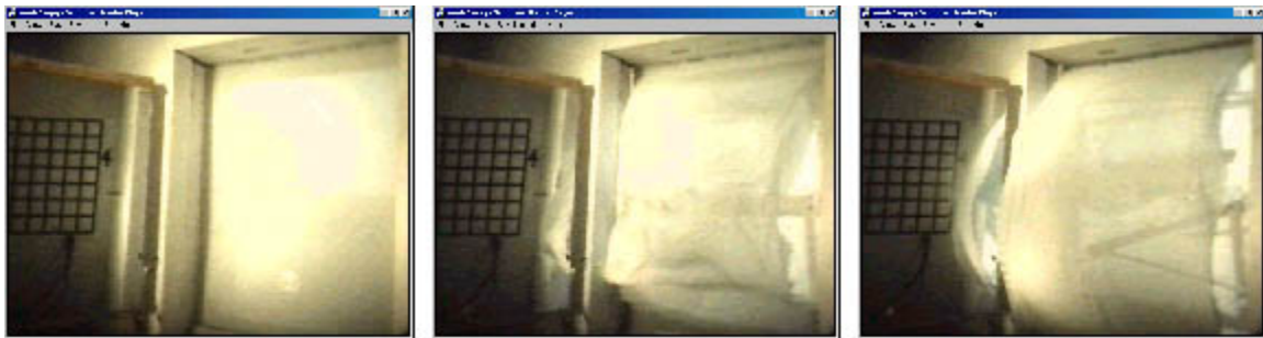
Blast Shield deploying under a blast load catches fragments and debris.
