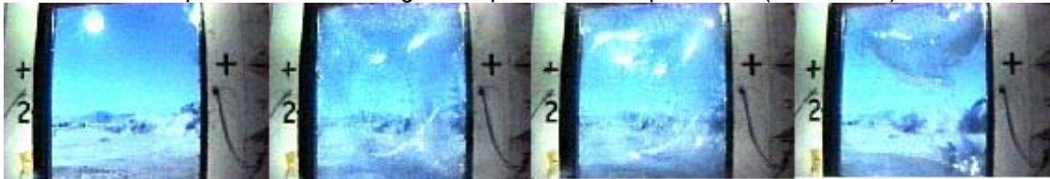
Security window film applied to annealed glass exposed to blast pressures (condition 3).
