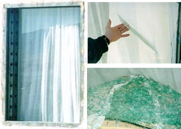
Blast Curtain pre- and post-explosion.
